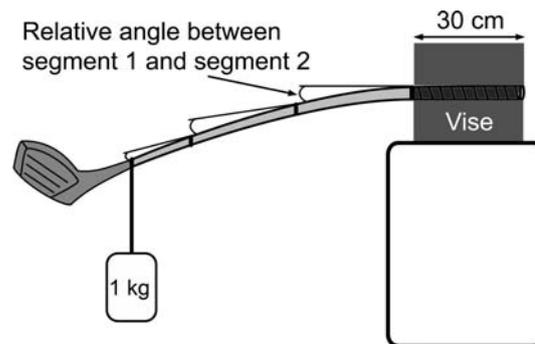
**Fig. 4** Experimental set-up for determining shaft stiffness
